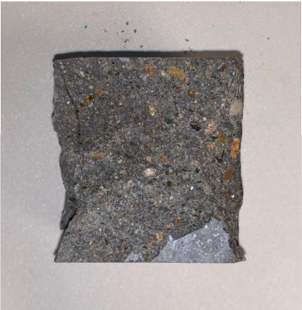
Photograph of an eco-concrete sample, after 7 days compressive strength testing
